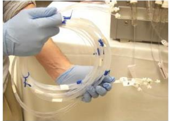
Customizable Teflon tubing with Luer locks
